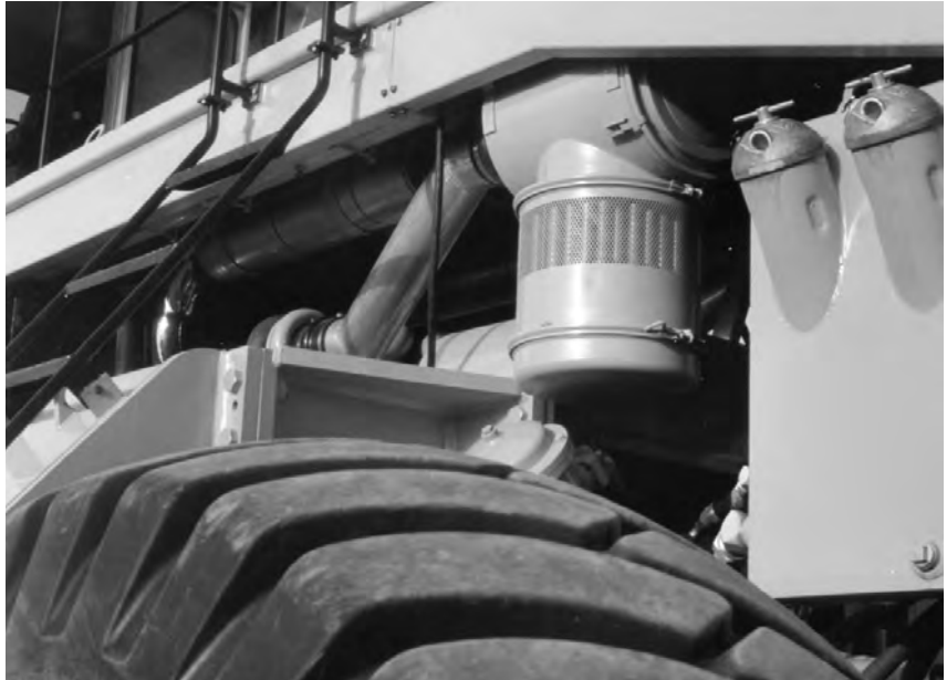
This STG Donaclone, mounted on a large mining machine, is protecting the engine from harmful dirt in this severely dusty environment.
