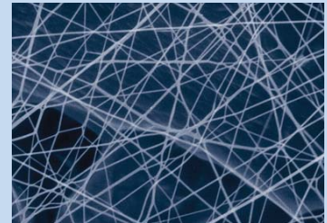
Scanning Electron Microscope image of Ultra-Web media magnified 1000 times.
