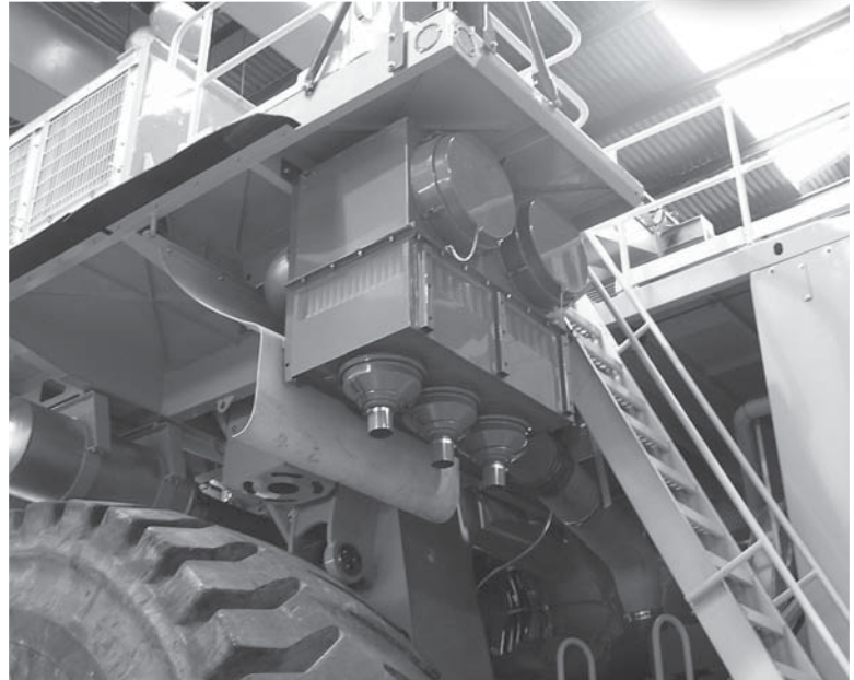
The large, massive mining vehicle in the picture above is an ideal match for the Donaldson SSG Air Cleaner.
