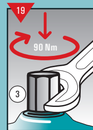
Tighten top nut with torque of 90 Nm
