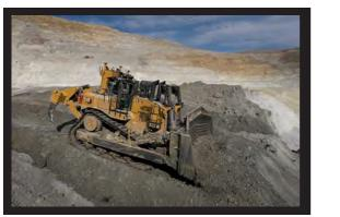
The new Cat D10 Dozer burns less fuel, increases productivity and improves uptime, says its maker. Featuring a stator clutch torque converter and loadsensing hydraulics, the new design is up to 6% more efficient than the Cat D10T2.
