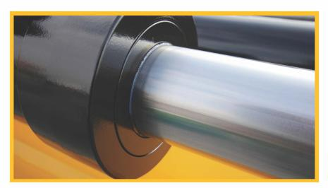
Effective hydraulic filtration is crucial in preventing damage to cylinders caused by hydraulic fluid contamination, which can result in wear, abrasion, and even catastrophic failure.
